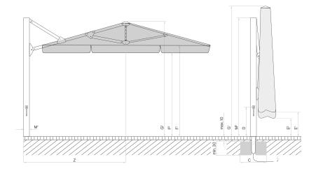
Loose cover max. 10 cm, concrete thickness min. 30 cm (pay attention to frost depth), guarantee water drainage, supply line electric.
