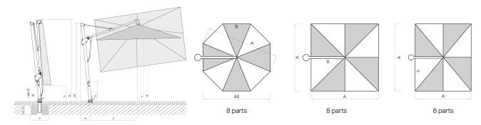
Loose cover max. 10 cm, concrete thickness min. 30 cm (pay attention to frost depth), Guarantee water drainage
